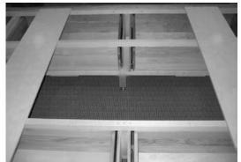
Attach a center support leg to the inside of each of the storage rails.
