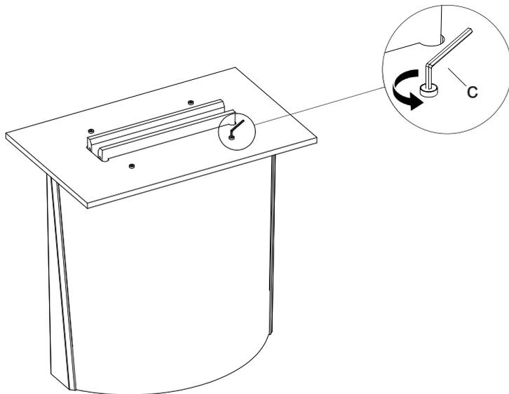
Use **allen key 'c'** to remove the protective top plate from the base. Save the washers ('a') and screws ('b'). You will need these when you attach the tabletop to the base.
