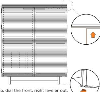
To move the right door up, dial the front, right leveler out. To move the left door up, dial the left, front leveler out.
