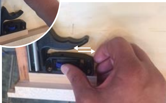
◇ Figure 3a. Level the drawer by adjusting the slides.
