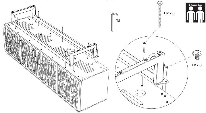
**Step 3 Triple -** With help from another person, carefully position the cabinet **A1** upside-down (as shown) or on its back. Attach the **base** to the **cabinet** with **8 Screws H1** and **6 Screws H2** using **Hex Wrench T2.** Do **NOT** fully tighten until all screws are started.
