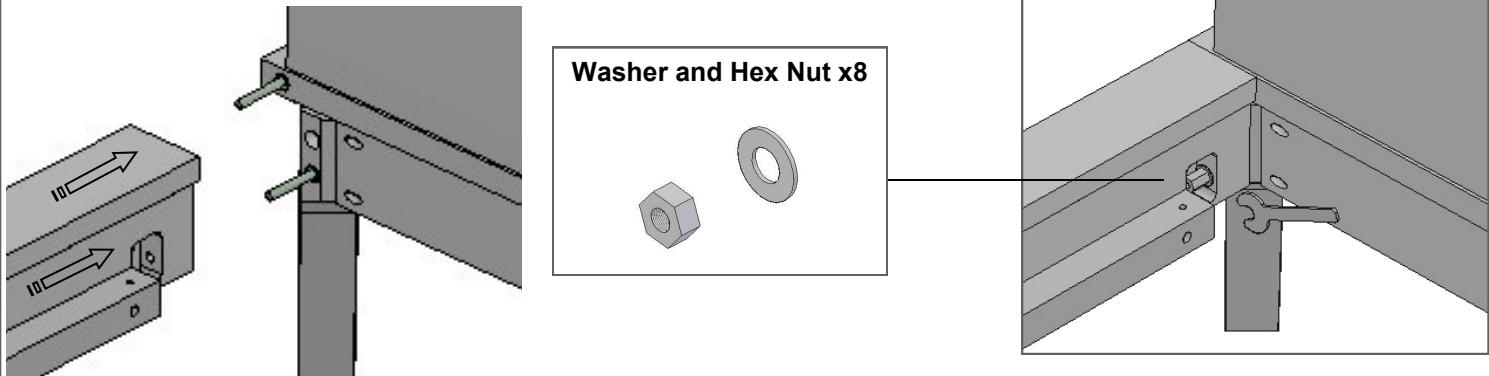
Slide a **side rail** onto the headboard using the dowel in the end of the rail and the threaded rod as a guide. Place a **washer and hex nut** over each rod. Fully tighten with the provided **straight wrench**.
