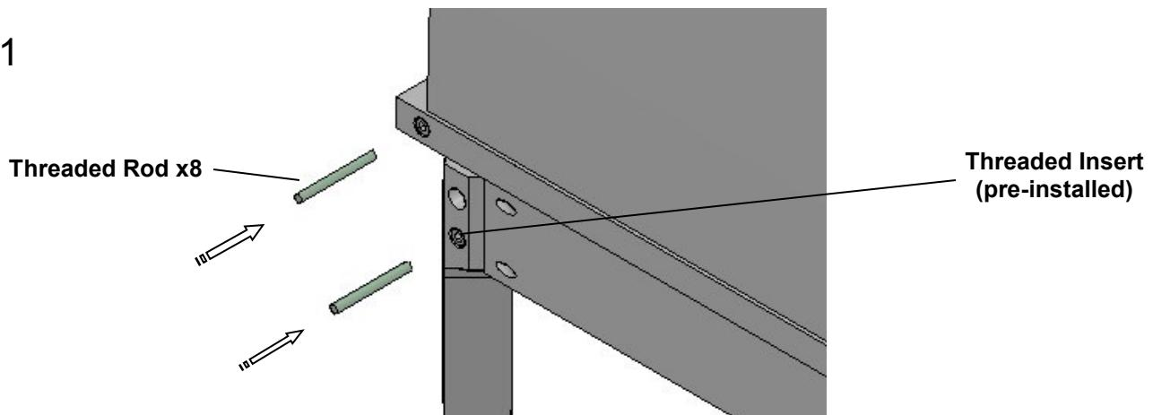
Install all **threaded rods** into the **threaded inserts** (pre installed in the headboard and footboard) and hand tighten as far as possible.
