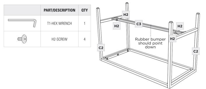
Attach the (C3) Lower Frame to the (C2) Legs using 4 (H2) Screws. Tighten with (T1) Hex Wrench.
