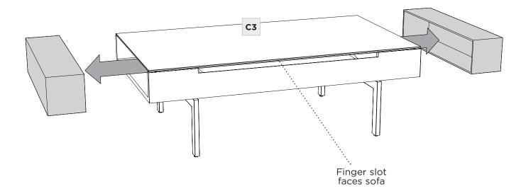
**NOTICE!** Objects placed in the indicated areas will interfere with the closing of the lift mechanism. Maximum height of objects in the center storage compartment should not exceed 2 1/2" | 64mm.
