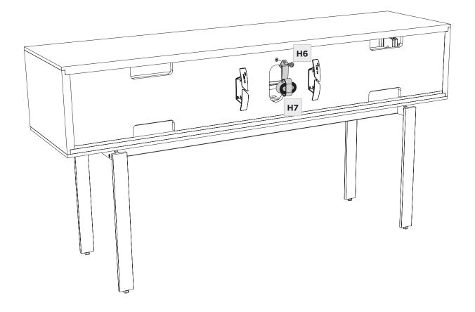
Make sure the console is level. Adjust one or more of the levelers using **(T2) Leveler Wrench**.
