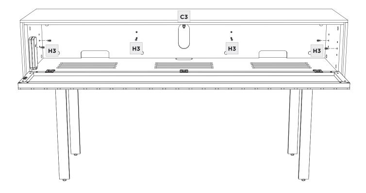
Carefully place the (C4) Glass Shelf into the (C3) Cabinet. Lift the shelf over the winch mechanism and gently lower it into position, resting on the shelf pins.
