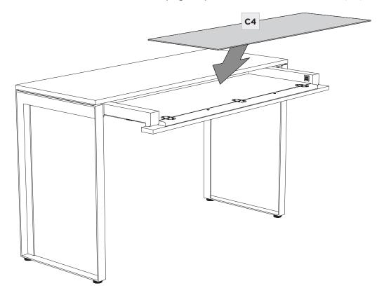
STEP 5. INSTALL WIRE MANAGEMENT EXTRUSION—OPTIONAL
