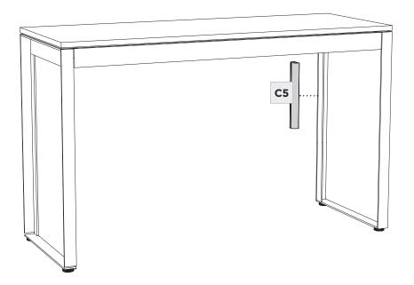
Your Linea Console is equipped with built-in levelers. Dial down one or more levelers (by hand) until you attain a level stance.
