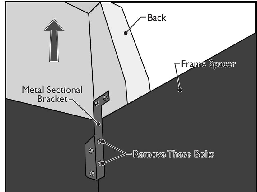
**Figure B.** Remove the two bolts pointed out in image above with a 1/2" socket. Do this for both sides of the back. With all four (4) bolts removed you can lift up the back and remove it from the comfort sleeper.
