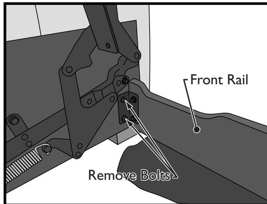
9. Remove the two bolts on each side of the comfort sleeper that secure the front rail to the arm. With the bolts removed, set the front rail aside.
