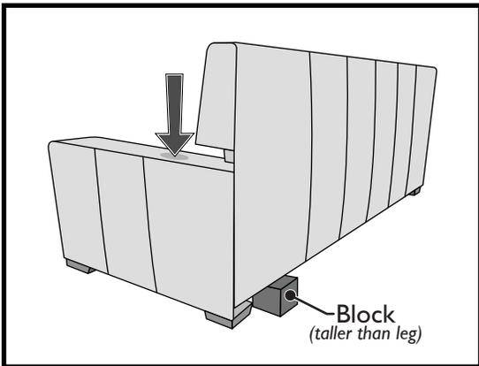
5. Turn the sofa upright and place a block (taller than the sofa leg) under the back near the arm. Press down firmly as shown in the figure above to release the arm from the back.
