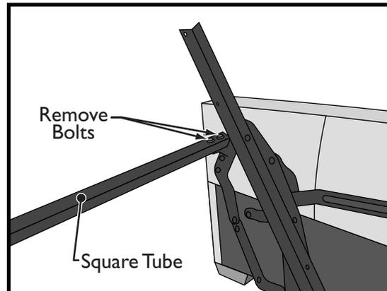
7. To remove the square tube, remove the two bolts on both sides of the comfort sleeper. With all (4) four bolts removed, set the square tube aside.
