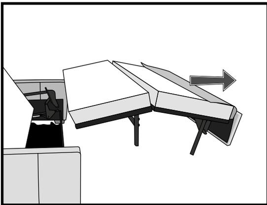
2. With the four (4) bolts removed, lift the front bed sections away from the comfort sleeper and set aside.
