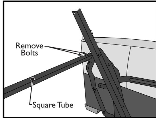
8. To remove the square tube, remove the two bolts on both sides of the comfort sleeper. With all (4) four bolts removed, set the square tube aside.
