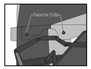
4. With the dustcover open, you have access to the bolts securing the back to the arms. Remove the two bolts, as shown in the figure above, from both sides of the comfort sleeper.
