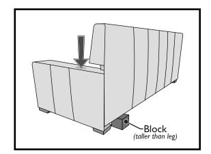
**5.** Turn the sofa upright and place a block (taller than the sofa leg) under the back near the arm. Press down firmly as shown in the figure above to release the arm from the back.
