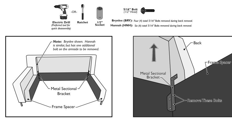
**Figure A.** Sectional Brynlee (BRY) and Hannah (HNH) comfort sleepers have a *frame spacer* on each side, as well as a *metal sectional bracket* on each side. The *metal sectional bracket* secures the back to the *frame spacers*.
