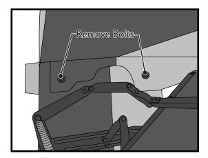
**4.** With the dustcover open, you have access to the bolts securing the back to the arms. Remove the two bolts, as shown in the figure above, from both sides of the comfort sleeper.
