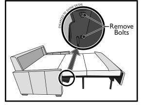
**I**. To begin, open the comfort sleeper as shown. Remove the two bolts connecting the middle bed section to the mechanism, as shown in the enlarged view. Do this on both the left and right sides.
