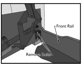
**8.** Remove the two bolts on each side of the comfort sleeper that secure the front rail to the arm. With the bolts removed, set the front rail aside.
