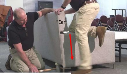
Place a 5" Block under the Back, near the Arm, and press down on the top of the Arm as shown to release the Back from the Arm on both sides of the sofa
