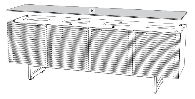
Place (K) Glass Top on top of (C) Cabinet. Position glass flush with cabinet front doors.
