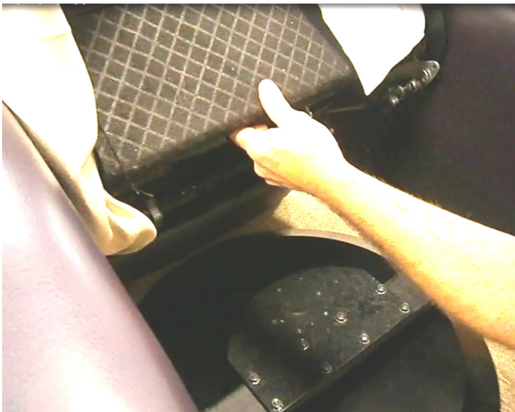
6. Pull the back of the Seat Frame to slide Tracks onto Shoes until they hit the Rubber Bumpers.
