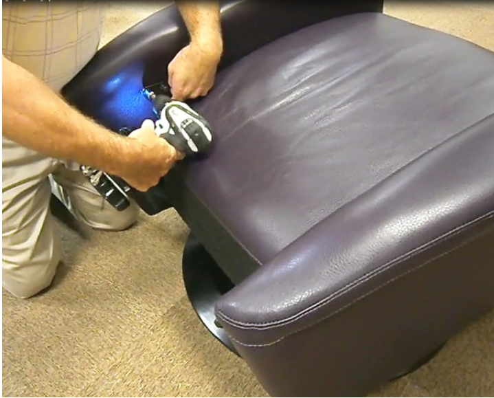
8. Start the two Bolts on each side by hand first and then tighten with the Drill.
